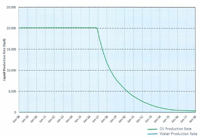
Note: Production profile is Base Case at 100% uptime for EPS phase of development. Actual production will be subject to uptime constraints, expecting to lead to plateau of 17,000 bopd. First production anticipated in H1 2019, not 2018 as indicated on chart.
